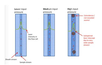
Pictures of increasing input pressure on data quality from MoFlo as example
