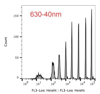
8peaks are small (3.5um) and very homogeneous: a well aligned instrument has CVs approx. 2% on the bright peak
