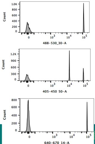
It is of very great use to test all your channels with 8peaks to see which channels (PMT/Filter combos) are your most dynamic!
